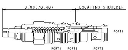
Direct-acting, 3-way directional cartridges (1 blocked, 2 to 3 open) are switching devices typically used in moderate flow circuits. They can be used by themselves or to actuate larger pilot-operated directional cartridges or logic cartridges. The valve shifts when the pressure differential between port 1 and port 4 exceeds the setting.
