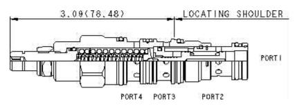
Direct-acting, 3-way directional cartridges (1 blocked, 2 to 3 open) are switching devices typically used in moderate flow circuits. They can be used by themselves or to actuate larger pilot-operated directional cartridges or logic cartridges. The valve shifts when the pressure differential between port 1 and port 4 exceeds the setting.
