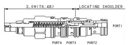
Direct-acting, 3-way directional cartridges (1 blocked, 2 to 3 open) are switching devices typically used in moderate flow circuits. They can be used by themselves or to actuate larger pilot-operated directional cartridges or logic cartridges. The valve shifts when the pressure differential between port 1 and port 4 exceeds the setting.
