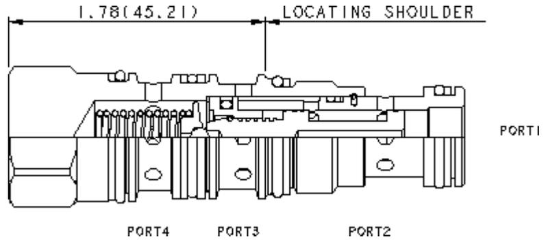
Direct-acting, 3-way directional cartridges (1 blocked, 2 to 3 open) are switching devices typically used in moderate flow circuits. They can be used by themselves or to actuate larger pilot-operated directional cartridges or logic cartridges. The valve shifts when the pressure differential between port 1 and port 4 exceeds the setting.
