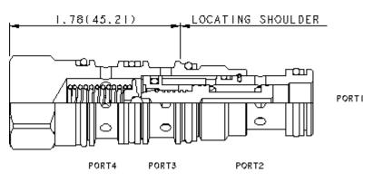
Direct-acting, 3-way directional cartridges (1 blocked, 2 to 3 open) are switching devices typically used in moderate flow circuits. They can be used by themselves or to actuate larger pilot-operated directional cartridges or logic cartridges. The valve shifts when the pressure differential between port 1 and port 4 exceeds the setting.
