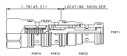
Direct-acting, 3-way directional cartridges (1 to 2 open, 3 blocked) are switching devices typically used in moderate flow circuits. They can be used by themselves or to actuate larger pilot operated directional cartridges or logic cartridges. The valve shifts when the pressure differential between port 1 and port 4 exceeds the setting.
