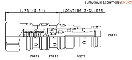
Direct-acting, 3-way directional cartridges (3 to 4 open, 2 blocked) are switching devices typically used in moderate flow circuits. They can be used by themselves or to actuate larger pilot operated directional cartridges or logic cartridges. The valve shifts when the pressure differential between port 1 and port 4 exceeds the setting.
