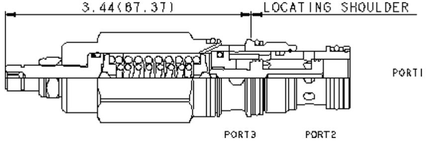
Direct-acting, 3-way directional cartridges (1 blocked, 2 to 3 open) are switching devices typically used in moderate flow circuits. They can be used by themselves or to actuate larger pilot-operated directional cartridges or logic cartridges. The valve shifts when the pressure differential between port 1 and port 3 exceeds the setting.
