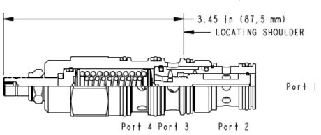
Direct-acting, 3-way directional cartridges (3 to 4 open, 2 blocked) are switching devices typically used in moderate flow circuits. They can be used by themselves or to actuate larger pilot operated directional cartridges or logic cartridges. The valve shifts when the pressure differential between port 1 and port 4 exceeds the setting.
