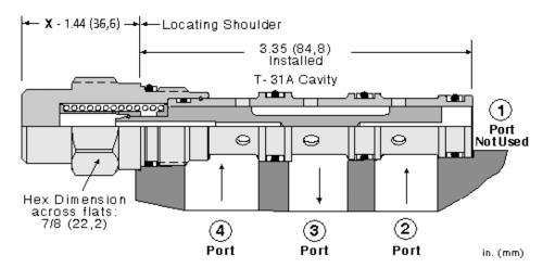
Low-side (hot oil) shuttle cartridges allow hot oil to be diverted from the low pressure side of a closed loop system. When both work ports (ports 2 and 4) are at equal pressures the valve is spring-centered to an all-ports-blocked position. When one of the work ports (port 2 or 4) sees a higher pressure the opposite work port is connected to the common port (port 3).
