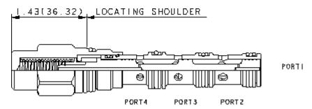
Spring-offset, high-side shuttle cartridges are 2-position valves that have a normal (offset) position that connects the common port (port 3) to work port 4, with work port 2 blocked. When the pressure at port 2 rises above the pressure at port 4, the cartridge shifts to connect the common port to port 2 with port 4 then blocked.
