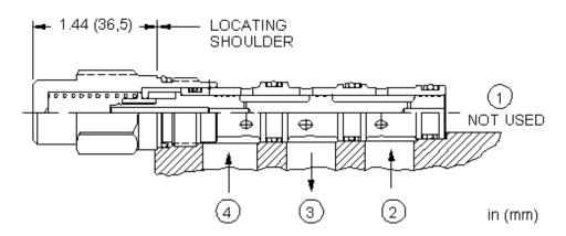
Spring-offset, high-side shuttle cartridges are 2-position valves that have a normal (offset) position that connects the common port (port 3) to work port 4, with work port 2 blocked. When the pressure at port 2 rises above the pressure at port 4, the cartridge shifts to connect the common port to port 2 with port 4 then blocked.
