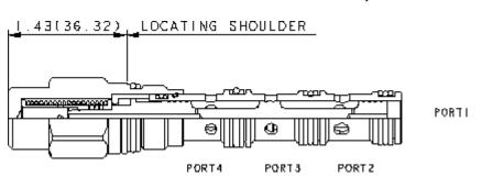
High-side shuttle cartridges are most often used in full-time regeneration circuits. When both work ports (ports 2 and 4) are at equal pressures the valve is spring-centered to an all-ports-blocked position. When one of the work ports (port 2 or 4) sees a higher pressure it is connected to the common port (port 3).
