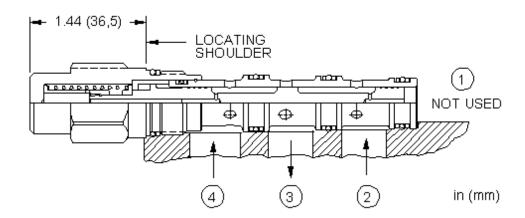
High-side shuttle cartridges are most often used in full-time regeneration circuits. When both work ports (ports 2 and 4) are at equal pressures the valve is spring-centered to an all-ports-blocked position. When one of the work ports (port 2 or 4) sees a higher pressure it is connected to the common port (port 3).
