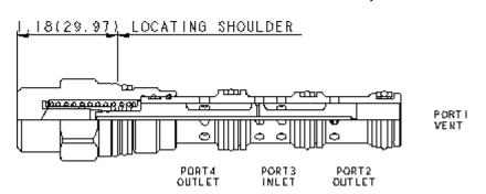
This is a vent-to-shift, 2-position, diverter valve that is normally closed. When port 1 is vented, the pressure
