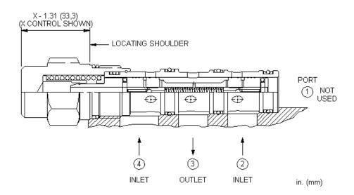
Low-side (hot oil) shuttle cartridges allow hot oil to be diverted from the low pressure side of a closed loop system. When both work ports (ports 2 and 4) are at equal pressures the valve is spring-centered to an all-ports-blocked position. When one of the work ports (port 2 or 4) sees a higher pressure the opposite work port is connected to the common port (port 3). The delay shift shuttle prevents flow transients downstream of the hot oil circuit.
