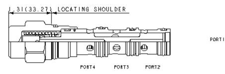
Low-side (hot oil) shuttle cartridges allow hot oil to be diverted from the low pressure side of a closed loop system. When both work ports (ports 2 and 4) are at equal pressures the valve is spring-centered to an all-ports-blocked position. When one of the work ports (port 2 or 4) sees a higher pressure the opposite work port is connected to the common port (port 3).
