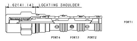
High-side shuttle cartridges are most often used in full-time regeneration circuits. When both work ports (ports 2 and 4) are at equal pressures the valve is spring-centered to an all-ports-blocked position. When one of the work ports (port 2 or 4) sees a higher pressure it is connected to the common port (port 3).
