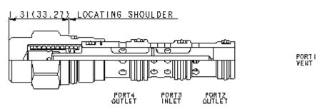
This is a vent-to-shift, 2-position, diverter valve that is normally closed. When port 1 is vented, the pressure differential between port 3 and port 1 exceeds the spring
