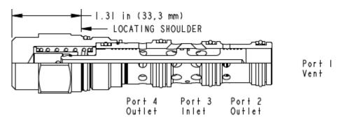
This vent-to-shift diverter valve is a 2-position, 3-way cartridge that is normally open from port 3 to port 4. When port 1 is vented, the pressure differential between port 3 and
