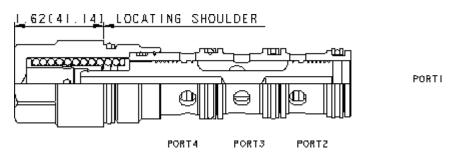
Low-side (hot oil) shuttle cartridges allow hot oil to be diverted from the low pressure side of a closed loop system. When both work ports (ports 2 and 4) are at equal pressures the valve is spring-centered to an all-ports-blocked position. When one of the work ports (port 2 or 4) sees a higher pressure the opposite work port is connected to the common port (port 3).
