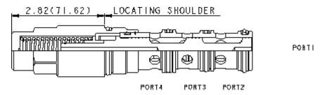
Spring-offset, high-side shuttle cartridges are 2-position valves that have a normal (offset) position that connects the common port (port 3) to work port 4, with work port 2 blocked. When the pressure at port 2 rises above the pressure at port 4, the cartridge shifts to connect the common port to port 2 with port 4 then blocked.
