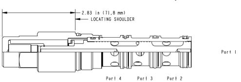
High-side shuttle cartridges are most often used in full-time regeneration circuits. When both work ports (ports 2 and 4) are at equal pressures the valve is spring-centered to an all-ports-blocked position. When one of the work ports (port 2 or 4) sees a higher pressure it is connected to the common port (port 3).
