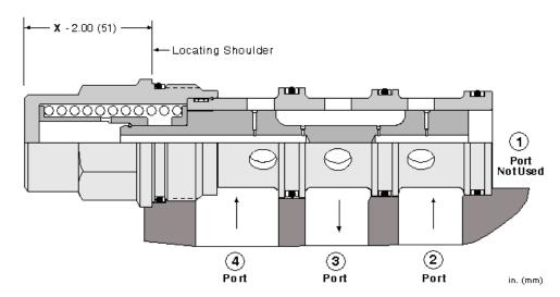
Low-side (hot oil) shuttle cartridges allow hot oil to be diverted from the low pressure side of a closed loop system. When both work ports (ports 2 and 4) are at equal pressures the valve is spring-centered to an all-ports-blocked position. When one of the work ports (port 2 or 4) sees a higher pressure the opposite work port is connected to the common port (port 3).
