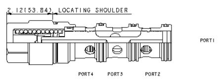
Low-side (hot oil) shuttle cartridges allow hot oil to be diverted from the low pressure side of a closed loop system. When both work ports (ports 2 and 4) are at equal pressures the valve is spring-centered to an all-ports-blocked position. When one of the work ports (port 2 or 4) sees a higher pressure the opposite work port is connected to the common port (port 3).
