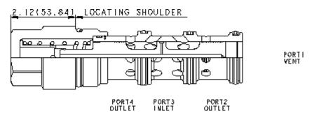
This vent-to-shift diverter valve is a 2-position, 3-way cartridge that is normally open from port 3 to port 4. When port 1 is vented, the pressure differential between port 3 and port 1 exceeds the spring force causing the valve to shift, thereby connecting port 3 to port 2.
