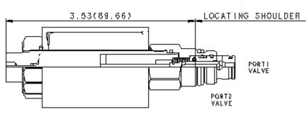
This FLeX Series solenoid-operated 2-way, 2-position cartridge is a direct-acting directional poppet valve. Available in either normally open or normally closed configurations, these valves feature a pressure-balanced design, low leakage, and allow flow or blocking in both directions. This cartridge can be installed directly into a cavity in the end of
