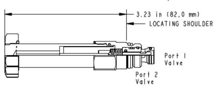
This FLeX Series solenoid-operated 2-way, 2-position cartridge is a direct-acting directional poppet valve. Available in either normally open or normally closed configurations, these valves feature a pressure-balanced design, low leakage, and allow flow or blocking in both directions. This cartridge can be installed directly into a cavity in the end of many of Sun's pilot operated and ventable valves to provide integrated pilot control.
