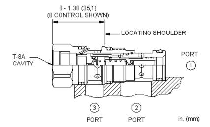
This valve is a normally open, 2-way directional cartridge that incorporates an integral pilot control cavity. It may be used by itself or to actuate larger pilot-operated directional cartridges or logic elements. The valve shifts when there is flow through the pilot control cartridge installed in the T-8A cavity.
