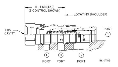
This valve is a normally open, 2-way directional cartridge that incorporates an integral pilot control cavity. It may be used
