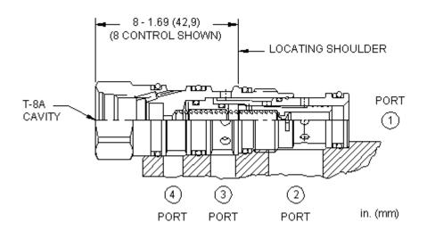
This valve is a normally open, 2-way directional cartridge that incorporates an integral pilot control cavity. It may be used by itself or to actuate larger pilot-operated directional cartridges or logic elements. The valve shifts when there is flow through the pilot control cartridge installed in the T-8A cavity.
