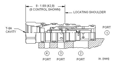
This valve is a normally closed, 2-way directional cartridge that incorporates an integral pilot control cavity. It may be used by itself or to actuate larger pilot-operated directional cartridges or logic elements. The valve shifts when there is flow through the pilot control cartridge installed in the T-8A cavity.
