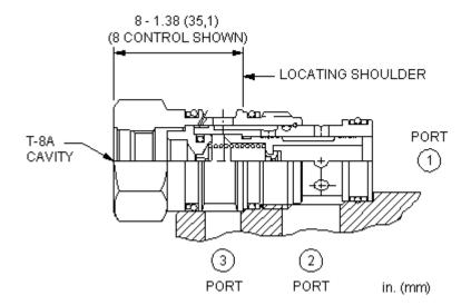
This valve is a normally closed, 2-way directional cartridge that incorporates an integral pilot control cavity. It may be used by itself or to actuate larger pilot-operated directional cartridges or logic elements. The valve shifts when there is flow through the pilot control cartridge installed in the T-8A cavity.
