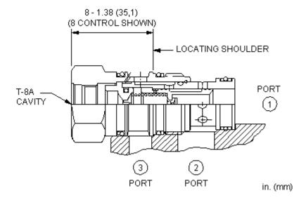
This valve is a, 3-way directional cartridge (1 blocked, 2 to 3 open) that incorporates an integral pilot control cavity. It may be used by itself or to actuate larger pilot-operated directional cartridges or logic elements. The valve shifts when there is flow through the pilot control cartridge installed in the T-8A cavity.
