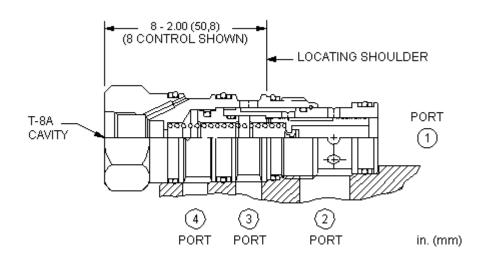
This valve is a normally open, 2-way directional cartridge that incorporates an integral pilot control cavity. It may be used by itself or to actuate larger pilot-operated directional cartridges or logic elements. The valve shifts when there is flow through the pilot control cartridge installed in the T-8A cavity.
