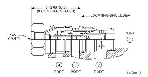
This valve is a, 3-way directional cartridge (1 blocked, 2 to 3 open) that incorporates an integral pilot control cavity. It may be used by itself or to actuate larger pilot-operated directional cartridges or logic elements. The valve shifts when there is flow through the pilot control cartridge installed in the T-8A cavity.
