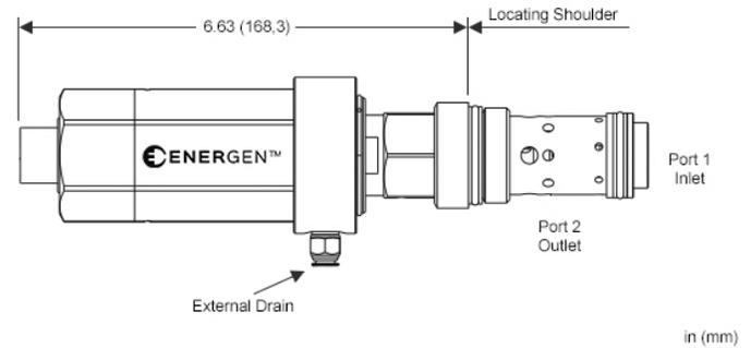
This valve is a 2 port cartridge designed to convert hydraulic power from your application into electrical power. The valve accepts flow from Port 1 to Port 2 and outputs a 3-phase AC voltage signal.
