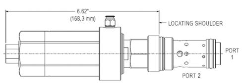
This valve is a 2 port cartridge designed to convert hydraulic power from your application into electrical power. The valve accepts flow from Port 1 to Port 2 and outputs a 3-phase AC voltage signal.
