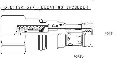
Fixed-orifice, pressure-compensated flow controls with reverse-flow check provide precise flow regulation for meterin or meter-out applications where there may be wide
