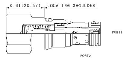
Fixed-orifice, pressure-compensated flow controls with reverse-flow check provide precise flow regulation for meter-in or meter-out applications where there may be wide pressure fluctuations. An integral high-capacity check valve provides unrestricted flow from port 2 to port 1. The flow setting is specified by the user and is set at the factory.
