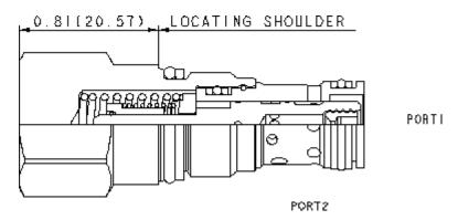
Fixed-orifice, pressure-compensated flow controls with reverse-flow check provide precise flow regulation for meterin or meter-out applications where there may be wide
