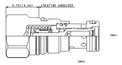
Fixed-orifice, pressure-compensated flow controls with reverse-flow check provide precise flow regulation for meter-in or meter-out applications where there may be wide pressure fluctuations. An integral high-capacity check valve provides unrestricted flow from port 2 to port 1. The flow setting is specified by the user and is set at the factory.
