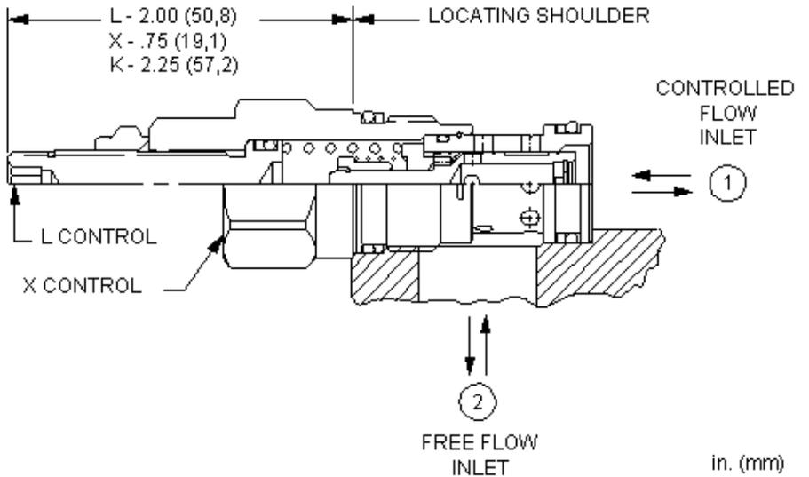
Fixed-orifice, pressure-compensated flow controls with reverse-flow check provide precise flow regulation for meter-in or meter-out applications where there may be wide pressure fluctuations. An integral high-capacity check valve provides unrestricted flow from port 2 to port 1. The flow setting is specified by the user and is set at the factory.
