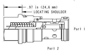
Fixed-orifice, pressure-compensated flow controls with reverse-flow check provide precise flow regulation for meter-in or meter-out applications where there may be wide pressure fluctuations. An integral high-capacity check valve provides unrestricted flow from port 2 to port 1. The flow setting is specified by the user and is set at the factory.
