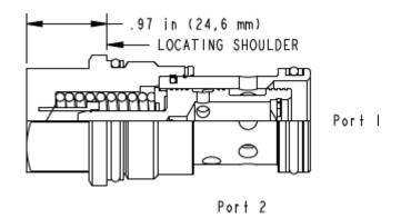
Fixed-orifice, pressure-compensated flow controls with reverse-flow check provide precise flow regulation for meter-in or meter-out applications where there may be wide pressure fluctuations. An integral high-capacity check valve provides unrestricted flow from port 2 to port 1. The flow setting is specified by the user and is set at the factory.
