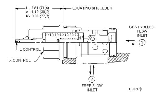
Fixed-orifice, pressure-compensated flow controls with reverse-flow check provide precise flow regulation for meter-in or meter-out applications where there may be wide pressure fluctuations. An integral high-capacity check valve provides unrestricted flow from port 2 to port 1. The flow setting is specified by the user and is set at the
