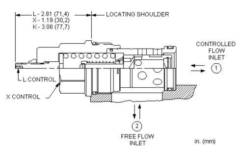
Fixed-orifice, pressure-compensated flow controls with reverse-flow check provide precise flow regulation for meter-in or meter-out applications where there may be wide pressure fluctuations. An integral high-capacity check valve provides unrestricted flow from port 2 to port 1. The flow setting is specified by the user and is set at the factory.
