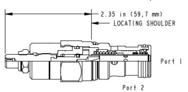
Fully adjustable, pressure-compensated flow controls with reverse-flow check provide precise flow regulation for meter-in or meter-out applications where there may be wide pressure fluctuations. They are infinitely adjustable from nearly closed up to the maximum flow. An integral high-capacity check valve provides unrestricted flow from port 2 to port 1.
