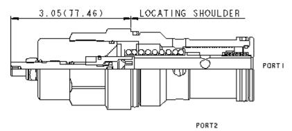
Fully adjustable, pressure-compensated flow controls with reverse-flow check provide precise flow regulation for meter-in or meter-out applications where there may be wide pressure fluctuations. They are infinitely adjustable from nearly closed up to the maximum flow. An integral high-capacity check valve provides unrestricted flow from port 2 to port 1.
