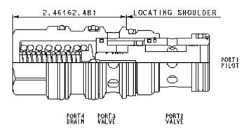
This valve is a 2-way, 2-position proportional throttle. Ports 2 and 3 are normally closed. Pilot pressure at port 1 creates a metering orifice between port 2 and 3 that is proportional to the pressure at 1. The force balance of the flow forces, spring and pilot pressure results in a degree of partial self-compensation as the load pressure changes. Pressure at port 4 directly opposes pressure at port 1.
