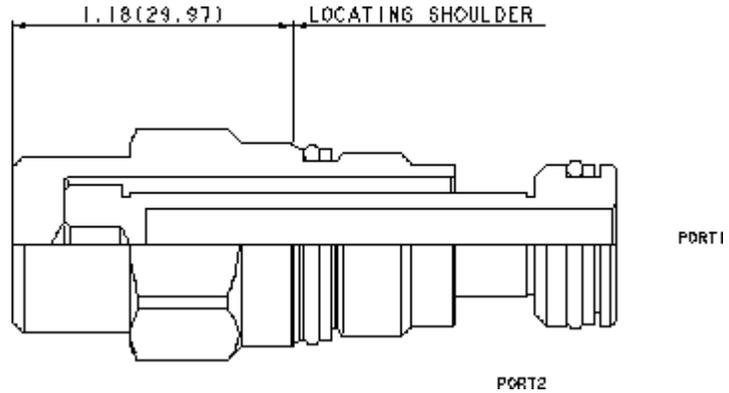
Sun filter elements are available as Surface Type (Last Chance) and Depth Style elements. The flow path is Port 2 to Port 1 and should not be used in reverse, even with a reverse free flow check valve installed. The elements have a high collapse pressure and are intended to be used in line with the system. Filter life will depend on initial system cleanliness and the amount of dirt ingress to the system when operating.
